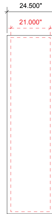
Finished Size: 24.5"w x 84.25"h Live Area: 21"w x 82"h Add 1.125" bleed on top and bottom of graphic Add 1.75" bleed on left and right side of graphic 1/2" Hook Velcro to be sewn into all 4 front sides.
